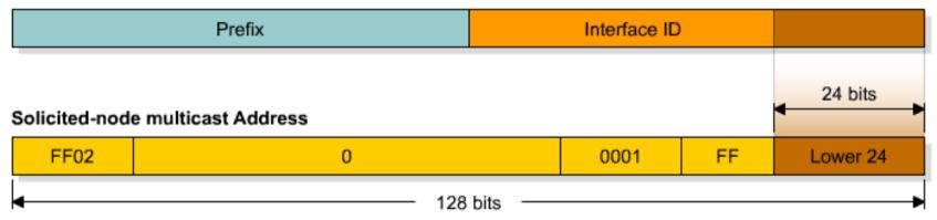
Solicited-node multicast address consists of FF02:0:0:0:0:1:FF::/104 prefix joined with the lower 24 bits from the unicast or anycast IPv6 address
