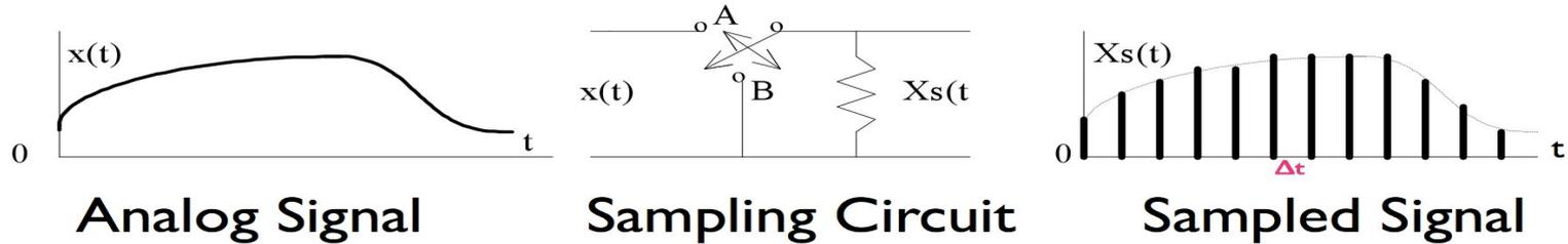
The sampling frequency  $f_s$  must be at least twice the highest frequency  $f_h$  present in the analog signal.
