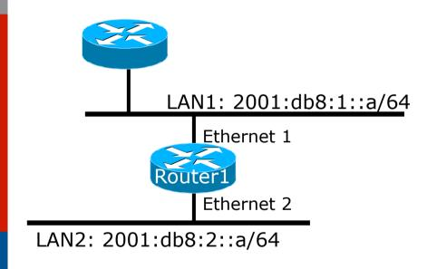
Dual stack IPv4/IPv6 configuration.
