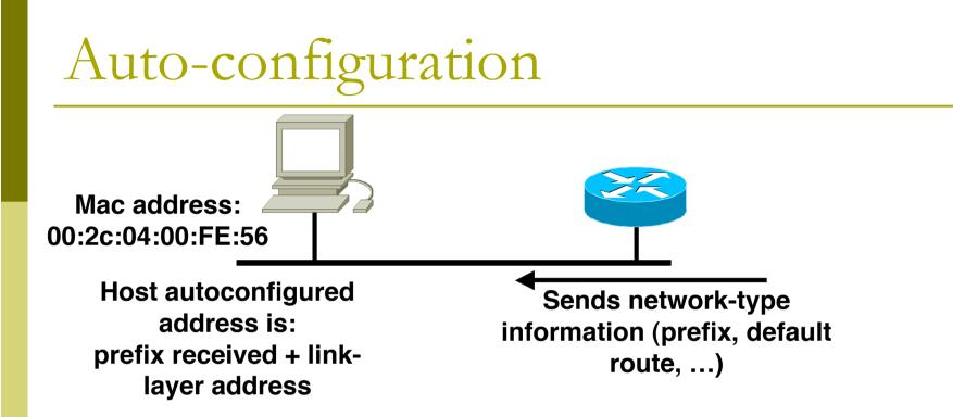
Client sends router solicitation (RS) messages Router responds with router advertisement (RA) This includes prefix and default route Client configures its IPv6 address by concatenating prefix received with its EUI-64 address
