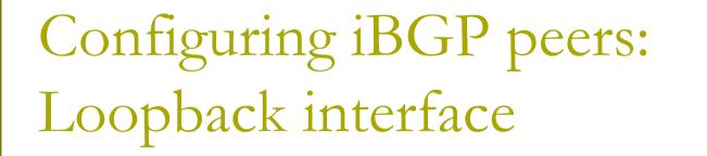
Loopback interfaces are normally used as the iBGP peer connection end-points
