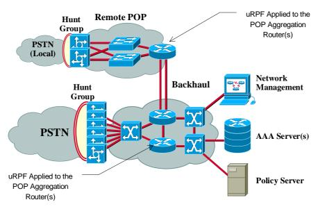
Figure 10 – Unicast RPF applied to PSTN/ISDN Customer Connections
