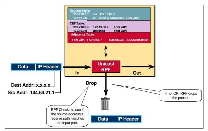
Figure 7 – Unicast RPF dropping packets which fail verification
