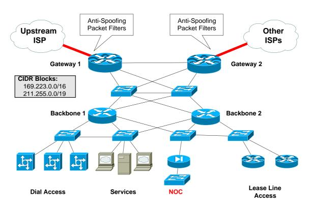
Figure 24 – Applying Anti-Spoofing Filters
