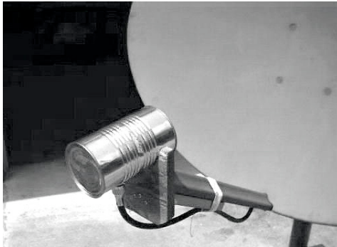
Figure 4.10: Feed horn made from a food can.
