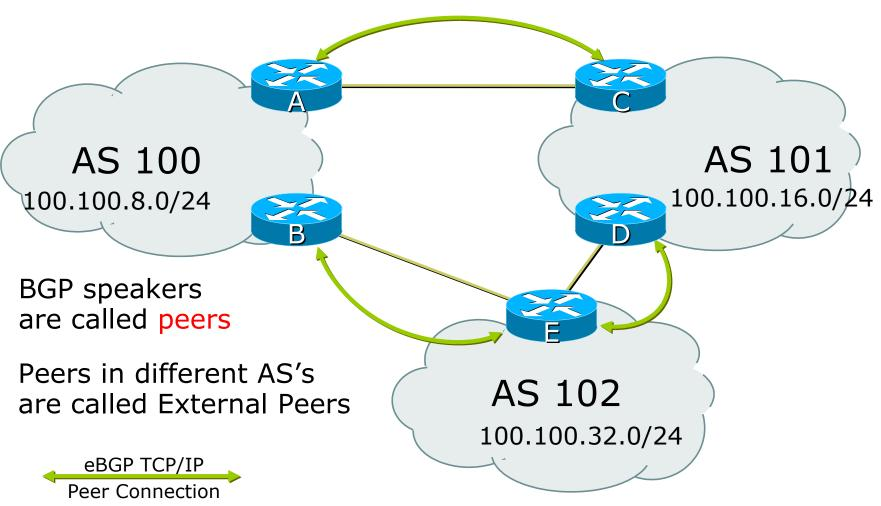
Note: eBGP Peers normally should be directly connected.
