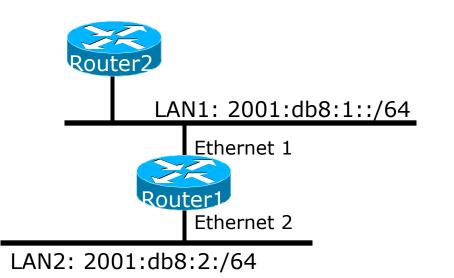
Dual IPv4/IPv6 configuration. Redistributing both IPv6 static routes and IPv4 static routes. Router1# interface ethernet 1 ip address 10.1.1.1 255.255.255.0 ipv6 address 2001:db8:1::1/64 ip router isis ipv6 router isis
