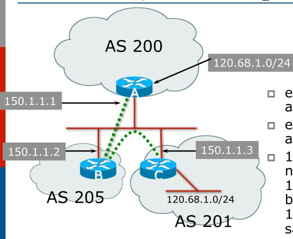
eBGP between Router A and Router B
