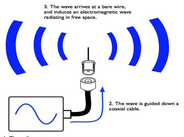
I. The radio creates an electrical current oscillating at high frequency.
