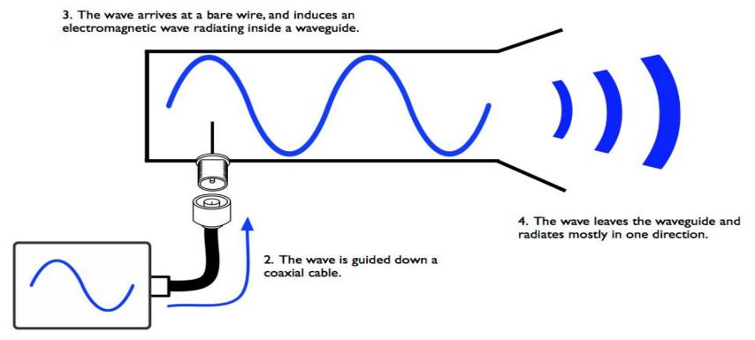
I. The radio creates an electrical current oscillating at high frequency.
